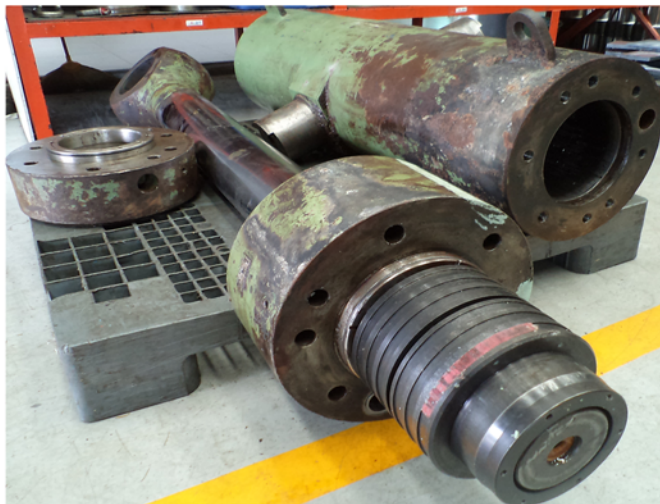
Hydraulic Cylinder Before Repair
